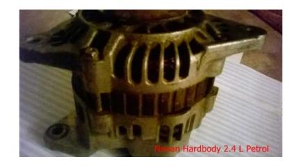
Will fit Nissan Diesel. Mounts on the left hand side of the engine. Genuine Nissan part in good working.
