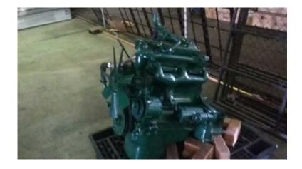
Mercedes Benz truck engine 508D (non turbo), complete engine & diesel pump have been over hauled by Automotive Engineering. Starts with.
