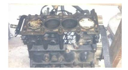
Audi agu motor, head striped of already have new headgasket, with 5speed gearbox
