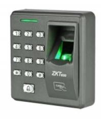
New ZKteco X7 fingerprint reader with RFID card reader built in. Small & elegant, electric lock control, doorbell button output, 500 prints, 500 cards, 12VDC, dimensions 88x88x33.6mm. For magnetic, striker & other electric.
