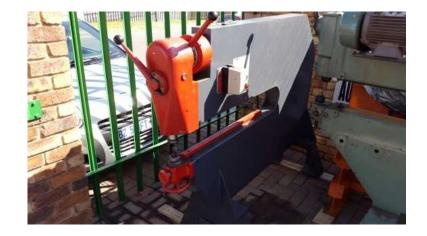
parts and panels , see pics for uses , first 2 pics are the machine other pics are just what these machines can do ,make ur own dies to suit each job ,run bead lines in floors ,flange edges,cut up to 7mm plate ,planish ,shrink steel,stretch steel,make any shapes ..etc etc all in one metal fabrication..
