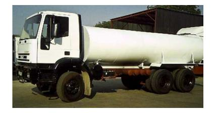
New mudguards and mud-flaps, new backboard with light, chevron board, New number plate light, underslung bumper, all reflectors and reflective tape, 5m piping and pump. Painted colour of your
